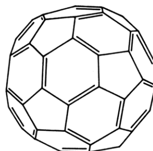
Figure 11. Proposed structure for the C_{60} cluster "buckminsterfullerene".
